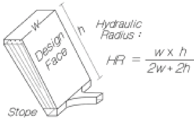
Figure 16.20: Hydraulic Radius Formula
