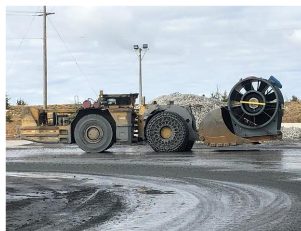
Eagle East main vent fan installation
