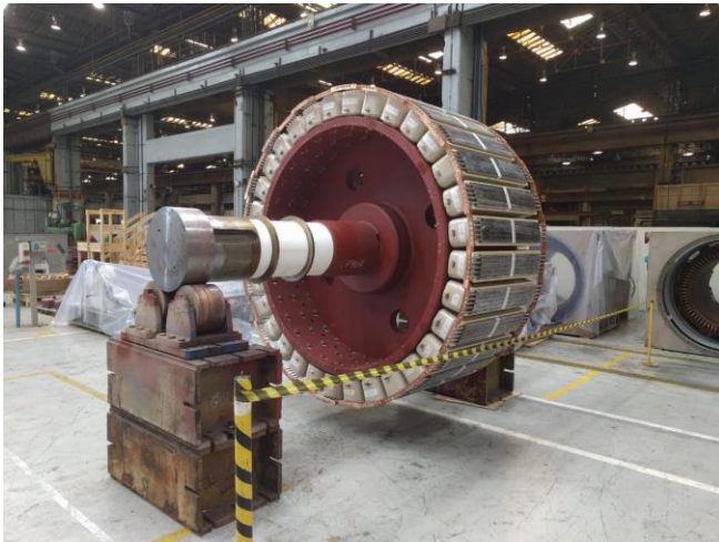
Ball mill motor replacements arriving on site
