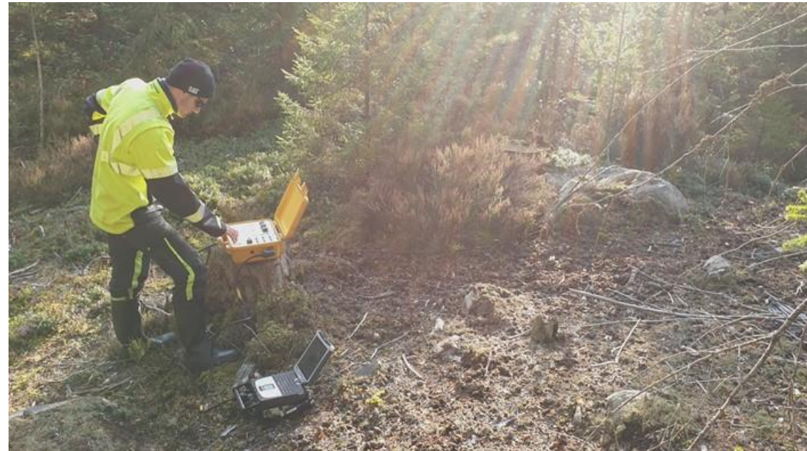
Zinkgruvan – October 2019 Ground EM Survey
