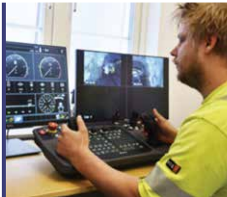
Remote operation of underground drill rigs, Zinkgruvan, Sweden.
