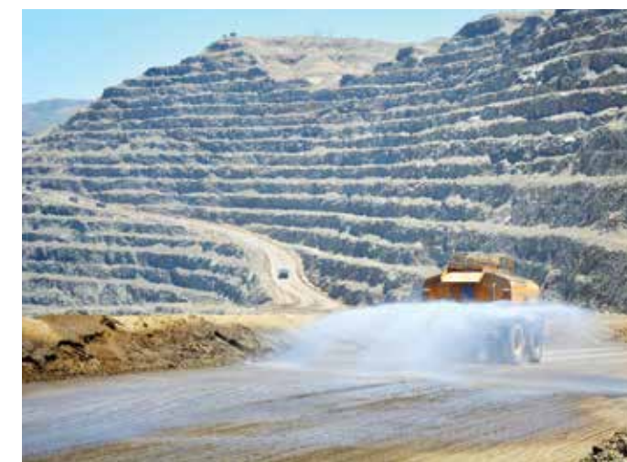
Dust Control Measures, Candelaria, Chile
